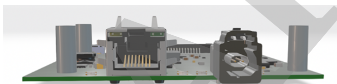
Figure 2: Ethernet connectors on Kvaser Arcus 100/1000BASE-T1 H-MTD
