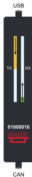
Figure 6: The TX LED bar lights up from the USB side to the CAN side of the unit, while the RX LED bar lights up from the CAN side to the USB side of the unit.
